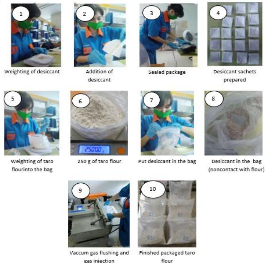
Figure 2. Packaging procedure for Beneng taro flour under modified-atmosphere conditions with densified dry bacterial cellulose.
