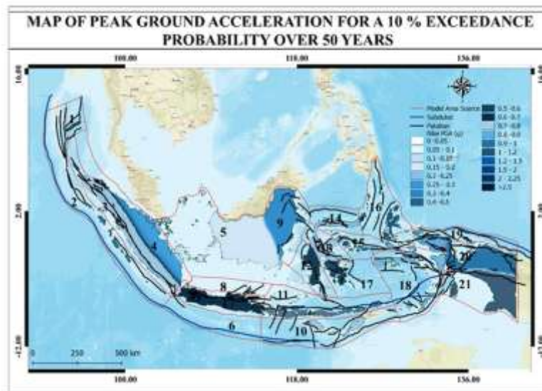
Figure 2. PGA Map for a 10% Exceedance Probability Over 50 Years (~475 years) Based on the Area Source Model
