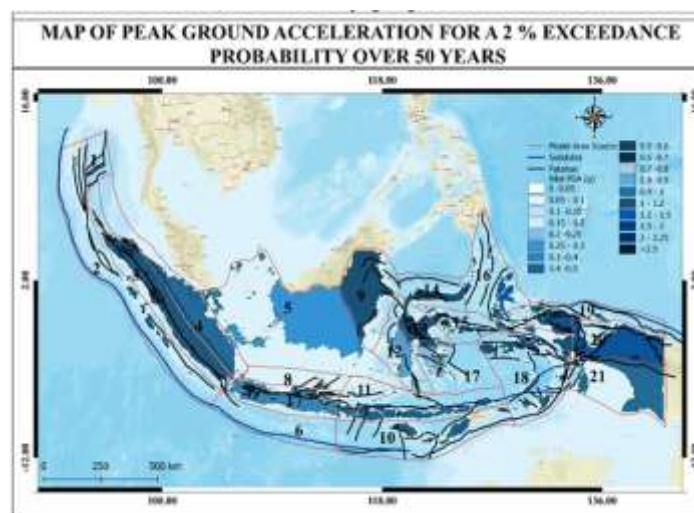
Figure 3. PGA Map for a 2% Exceedance Probability Over 50 Years (~2475 years) Based on the Area Source Model
