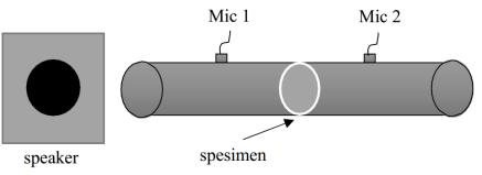
Figure 2. Testing technique using the tube method
