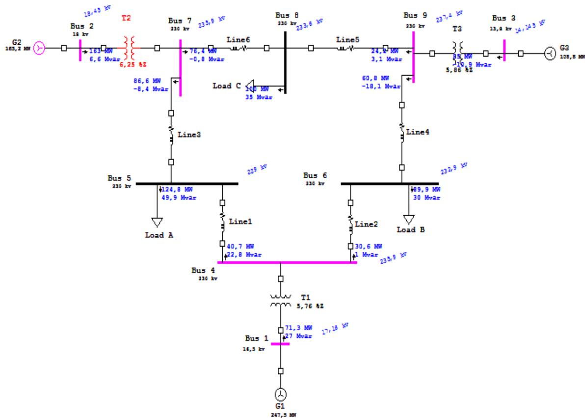
**Figure 4.** Single line diagram load flow results
