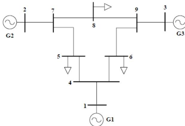
Figure 3 Single line diagram of 9 buses
